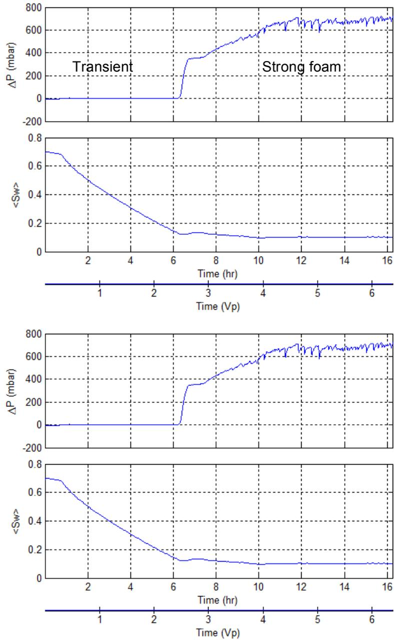
Figure 3: Generation of foam at a low interstitial velocity (1 ml/h, 1.6 cm/h). See text for explanation. Clashach sandstone, porosity 20.2%, 1550 mD,  $f_g=0.6$ , brine 35 gr/l, AOS type surfactant concentration 0.5 wt%.
