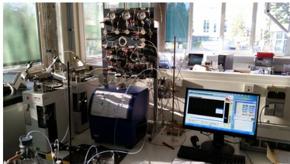
Figure 2: Schematic of the experimental set-up using NMR imaging. Gas controller (G.C.): controller to impose a fixed gas flow rate. Back pressure regulator (BPR): used to set the outlet pressure. The MRI system is a 20 MHz compact permanent magnet system from Oxford Instrument.
