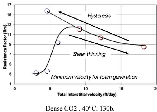
Figure 1: Typical behavior of foam when increasing the total interstitial velocity. An hysteresis may occur with decreasing velocity, yielding higher resistance to gas far from the well (Nabzar, 2014, ADRAAC, Abu Dhabi).
