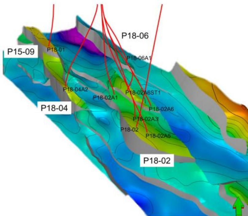
Figure 2: 3D view on the top of the P18 gas fields. Faults are shown in grey; well traces are shown in red (Arts et al., 2012).
