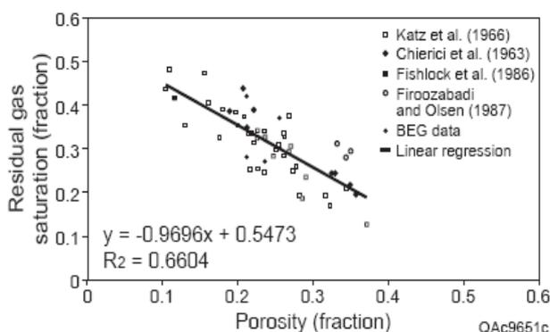
Figure 8: Different experimental data relating porosity to residual gas saturation.
