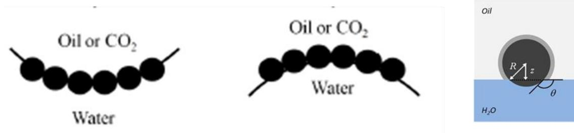
Figure 12: Interfacial adsorption of emulsion by solid nanoparticles.
