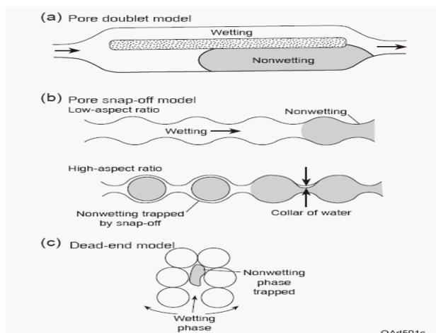
Figure 7: Three conceptual trapping models.
