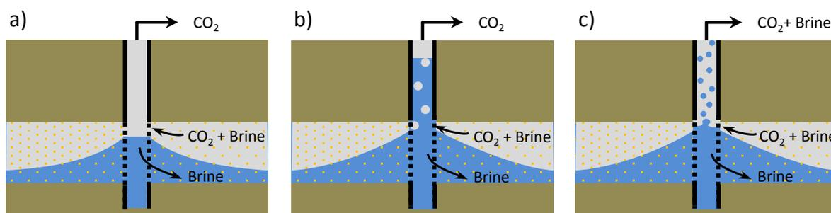
Figure 11: Three operational modes during the back production test.
