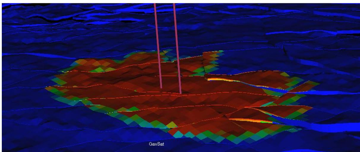
Figure 4: CO<sub>2</sub> saturation profile at the end of the injection.
