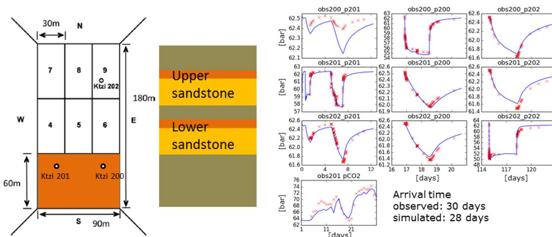
Figure 1: Simple inverse reservoir model including single phase hydraulic data, multiphase injection pressure and arrival time. The orange regions show sandstone areas with high permeability that act as channels for preferential CO<sub>2</sub> flow.
