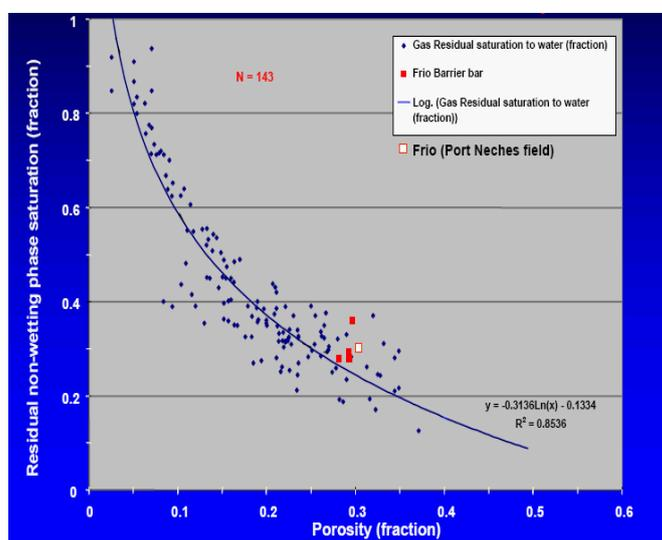
Figure 10: Residual gas saturation vs porosity (Holtz, 2005).
