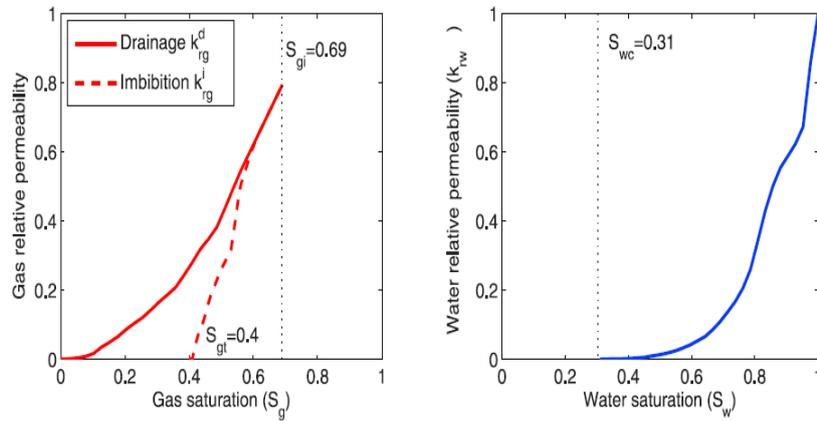
Figure 5: Relative permeability (water-wet Berea sandstone).
