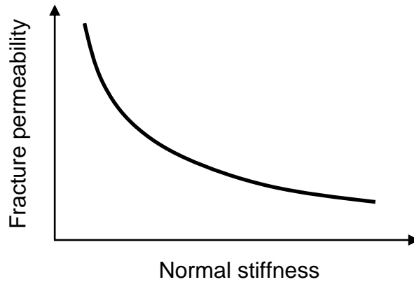
Figure 2.9 Fracture permeability versus normal stiffness under applied normal stress, after (Pyrak-Nolte, 1996).
