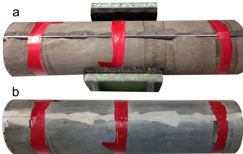
Fig. 1. Sample 1 - cement sample with a steel plate: (a) Half-cylinders reassembled with a steel plate; (b) Rough edges of the cement halves were filled with plaster and surface was polished.
